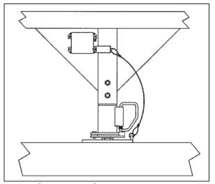
Breakaway Brake Connection - Figure 3-12
