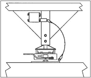
Breakaway Brake Connection - Figure 3-18
