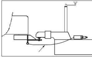
Breakaway Brake Connection - figure
