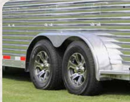
Aluminum construction of Sooner Select trailers features stout, durable triple hollow core sidewalls. The trailer is built with 2" x 4" I-beams on 13" centers, meeting the demands of transporting livestock across the country.
