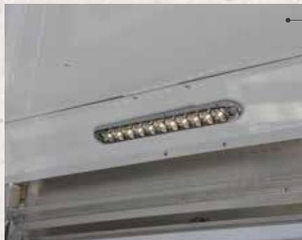
The Sooner Select features a bright LED light strip that alternates every 2 pens on each side, allowing for more consistent lighting throughout the interior of the trailer.
