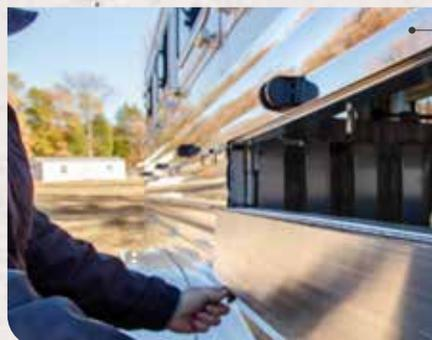
Lower air gaps with hinged cover panels on models with drop down windows allow for more air movement directly on the livestock.
