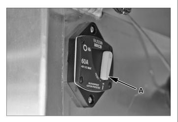
There are several replaceable blade type automotive fuses on the circuit panel. There is a circuit breaker that powers the 12 volt panel. Check this breaker if all 12 volt circuits are out.
