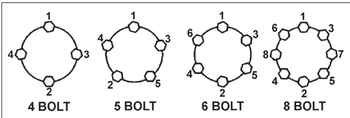
*Lug Nut Sequence of Tightening - Figure 8-8*
